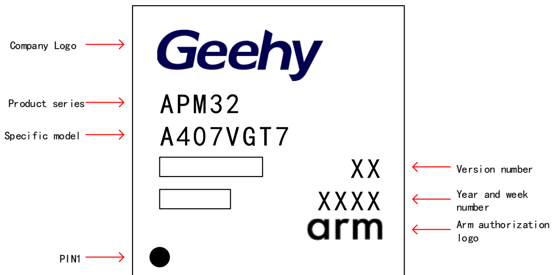
Figure 19 LQFP100 - 100 Pins, 14 x 14mm Package Schematic Diagram
